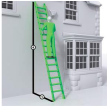
Figure 1 Ladder showing the correct 1 in 4 angle (means of securing omitted for clarity)
